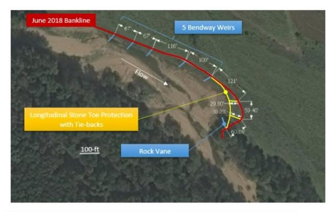
1. 5 Bendway Weirs (480-tons) to control conveyance of flow energy 2. Longitudinal Stone Toe Protection (360-tons) with Tie-backs (350-tons) to convey flow through a mild bend. (400-cy of onsite gravel to fill area between toe rock, tie-backs and bank) 3. Rock Vane (60-tons) to control exit conveyance
